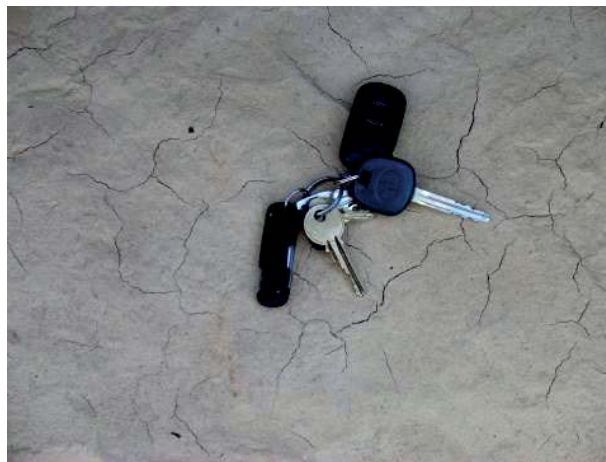
Figure 1-1: Plastic shrinkage cracking of concrete (concretenetwork.com)
