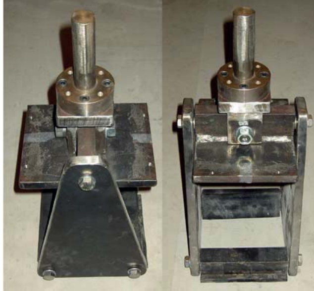
Figure 4 – Custom-welded self-centring anchor clamps
